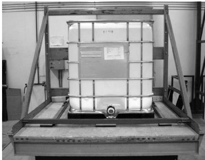
FIG. 1 Intermediate Bulk Container Test Specimen on Vibration Machine
